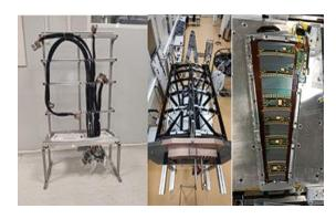
ATLAS ITk upgrade: connectorized cables in the service module (left), service module assembled into the mock-up of the global structure used for the system tests (center) and pre-production petal loaded with 9 modules on each side (right).
