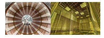
Left: the NEXT-100 TPC installed at the LSC, before closing the pressure vessel. Right: the ProtoDUNE-VD 4x6x6 m³ Time Projection Chamber at CERN, with visible PDS modules (60x60 cm2 at the top).
