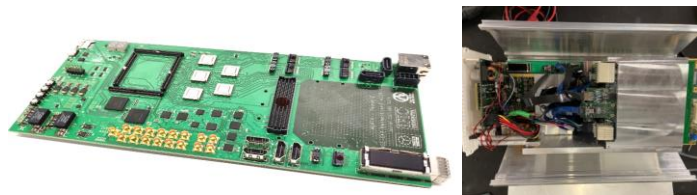
Left: Pre-processing motherboard PACE-CAP developed for AGATA at IFIC and ETSE. Right: Cooling mechanics with heat-exchanger and cooling blocks, built at the IFIC mechanical workshop.
