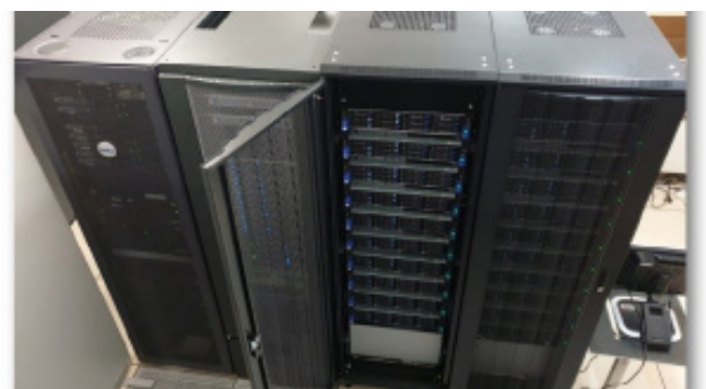
Front view of Artemisa (the three rightmost racks). The rack in the centre (open door) contains the GPU units
