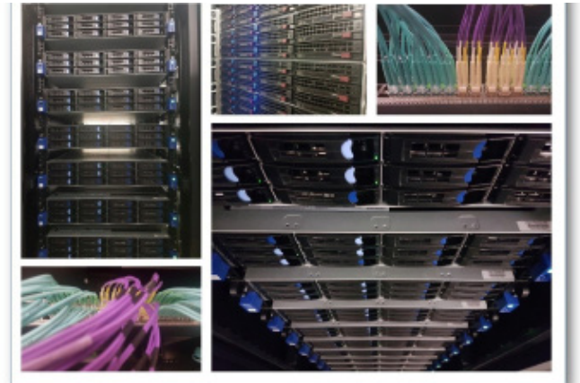
Photo collage of the equipment that composes Artemisa. Top left and bottom right: GPU units; Top centre: storage disks; Top right and bottom left: network switcher cables.
